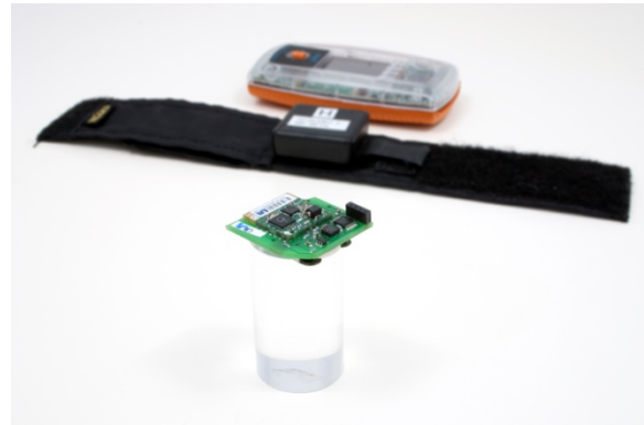
Sensors with velcro for attachment to the patient and the portable data logger.
